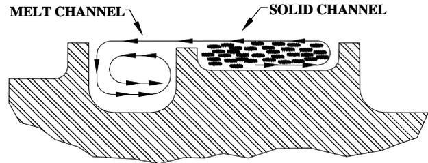
Figure 3. Barrier screw channel flow.
