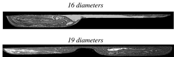
Figure 5: Channel cross sections for the ET extruder screw (9). The white regions are un-melted resin while the gray regions indicate molten and well mixed resin.
