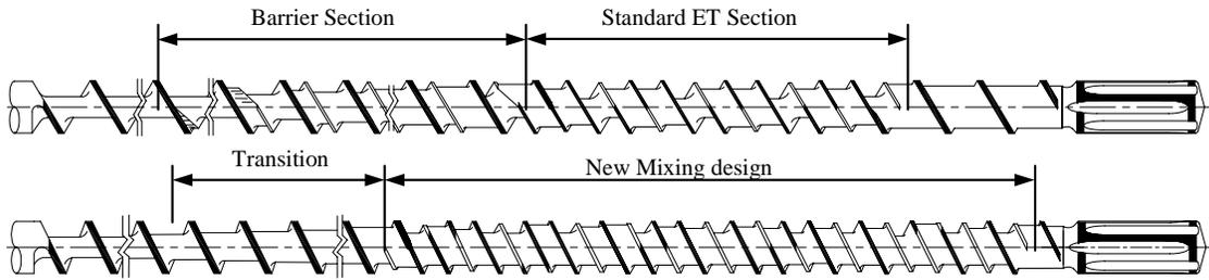
Figure 7. Standard barrier ET vs. New design.
