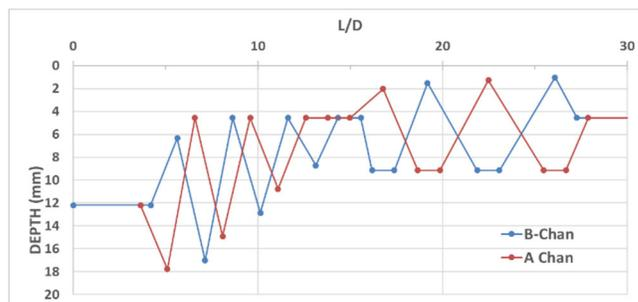
Figure 6. 63.5 mm, 33 L/D VBET-NSB channel profile.
