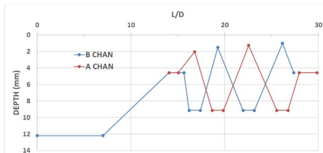
Figure 5. 63.5 mm, 33 L/D VBET channel profile.
