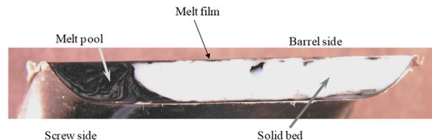
Figure 1. Photograph of resin solidified in the transition section after a Maddock solidification experiment for an ABS resin [3]. The pushing flight is on the left side of the photograph. The white material (with a black masterbatch) was solid when the screw was stopped, and the black material was molten.
