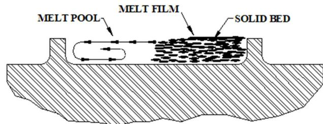
Figure 2. Schematic of the melting process in a conventional screw transition section.
